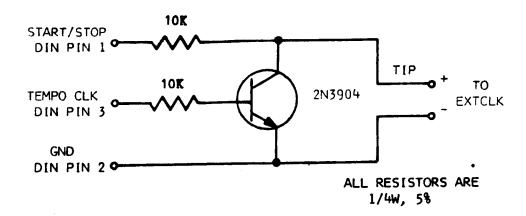
The sync switch on the Roland TR606 and TR808 should be set to OUT since it will be the master. Pins 4 and 5 of the DIN connector are not used. This circuit could be mounted inside a custom-built cable. The slow speed of the TR606 and TR808 and the clock inversion of this circuit may cause undesirable delays.
