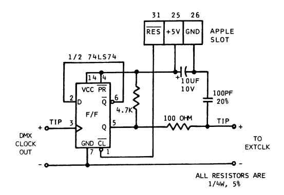
The Roland TR808 and TR606 (4) present a more complex problem, but an easier solution. The clock signal is not gated. Instead, the clock is free running and a start/stop signal is provided. It is possible to gate the free running clock with the start/stop signal, providing a compatible clock signal. The following circuit should work:
